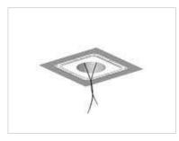
**STEP 3** Position the fixture by using a laser and the alignment marks
