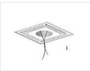
**STEP 2** Glue and screw the fixture against the surface
