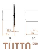
fixed (AR70) 30° tilt -360° (LED 0 50 mm) see accessories below excluded, except for Xillo Tube 0 80 mm 0 44 mm plasterboard (PB): 204 x 204 mm concrete (CC): 0 101 mm plasterboard (PB): 95,5 mm concrete (CC): 102 mm
