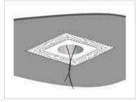
**STEP 4** Fill gaps with joint filler
