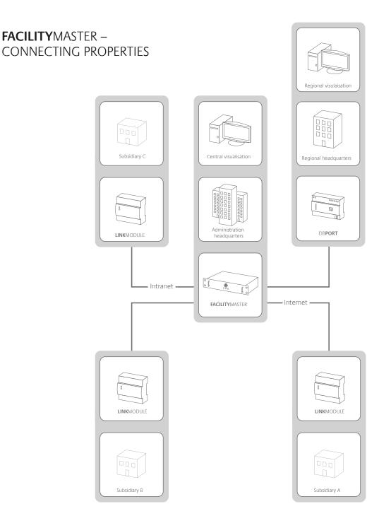
The **FACILITY**MASTER sits at the company's headquarters as a central manager. The properties are connected using communication technology via the Internet or the Intranet. Thanks to encoded Unicast communication, data transfer is secure and can be established without taking any further measures. For larger properties where own services and visualisation are required, the EIB**PORT** is used as a coupler. The **LINK**MODULE is used for smaller properties (e.g. warehouses, etc.).
