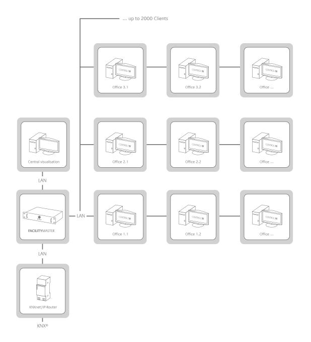
The **FACILITY**MASTER is installed centrally in the network and administrates the CONTROL **W**-visualisations for all clients connected (up to 2000). The high-performance hardware executes up to 2000 services reliably. Additionally, central visualisation is available which depicts the global system status. The connection to KNX<sup>®</sup> takes place via the network and KNXnet/IP.
